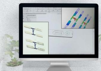
The simulations carried out before the mould insert is produced enable a well-founded assessment of the expected performance in the subsequent injection moulding process.
